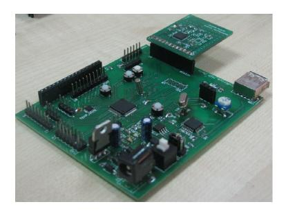
Snapshot of Zigbee based ultra-low power Wireless Sensor Network Development platform
